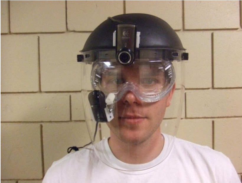
Figure 4: Eye tracker being worn
